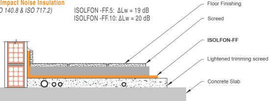
ISOLFON-FF application in floating concrete floor.
