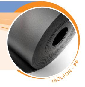
ISOLFON-FF is easy installed in a great range of applications where impact noise insulation on floating floors is required. It is produced from Expanded polyethylene cross linked foam, with density of about 28 kg/m<sup>3</sup>, which takes the shape of a rolled sheet. The structure of closed cells offers a greater deflection and rebound (after tension and release) due to the fact that air is trapped in the cells. Additionally it offers perfect resistance in water and humidity absorption.
